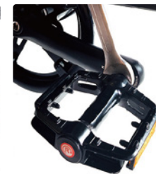
Tighten the left pedal "L" counter clockwise
