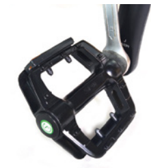
Tighten the right pedal "R" clockwise
